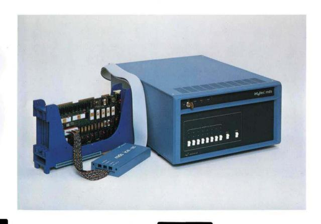
With the powerful Intellec MDS Microcomputer Development System and its ICE-80 In-Circuit Emulator, you can develop and debug your system software directly on the SBC 80/10 ... plus, you can isolate and correct system "bugs" on the production line and in the field
