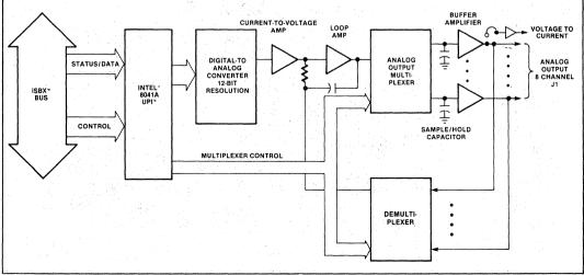
Figure 1. iSBC 328 Analog Output MULTIMODULE Board Block Diagram
