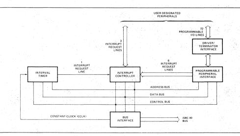
Figure 1. iSBC 519 Programmable I/O Expansion Board Block Diagram
