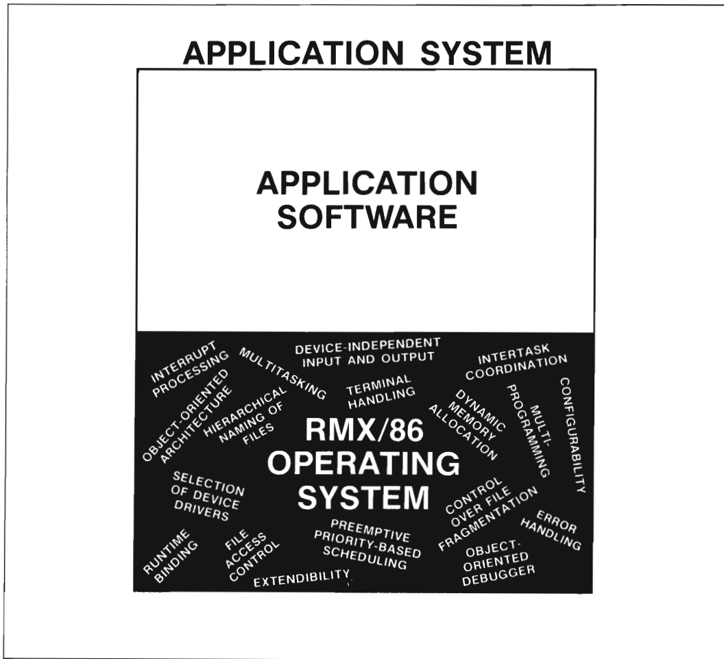
Figure 4-1. Features of the RMX/86 Operating System.
