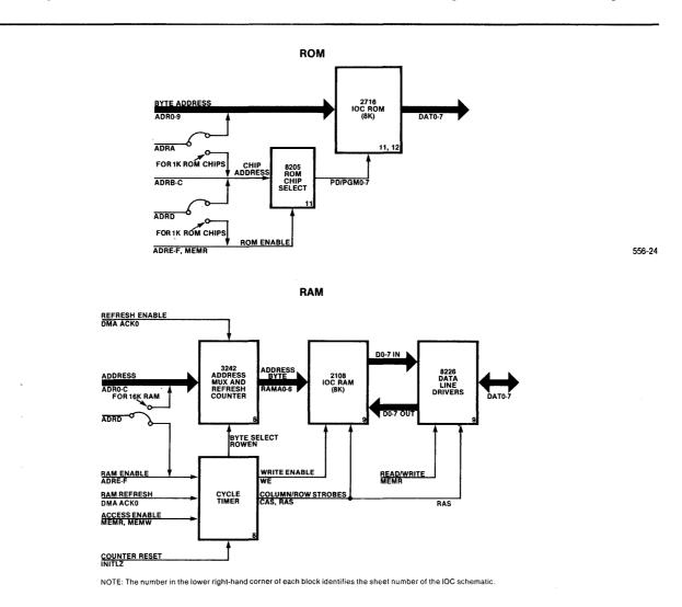
Figure 4-3. IOC Memory Subsystem Block Diagram
