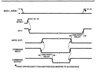
Figure 2-4. Bus Control Cycle Timing 556-7
