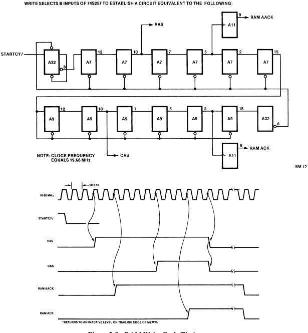
Figure 2-8. RAM Write Cycle Timing
