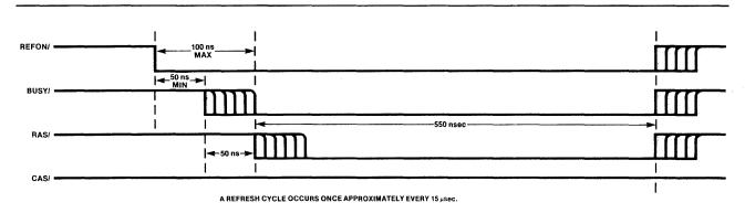
Figure 2-6. RAM Refresh Cycle Timing
