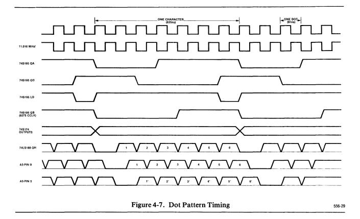
retrace intervals. These latter variables are established by values sent to the CRT controller when it is initialized. Associated hardware timing circuits control sweep triggering during the retrace intervals. These hardware timing circuits include the 8253 interval timer and the 74S195 shift register of the CRT dot generator. Both the programmed and the hardwarecontrolled variables are determined by the presence or absence of the 50 HZ JUMPER (W8). Sweep timing is shown in figure 4-8.
