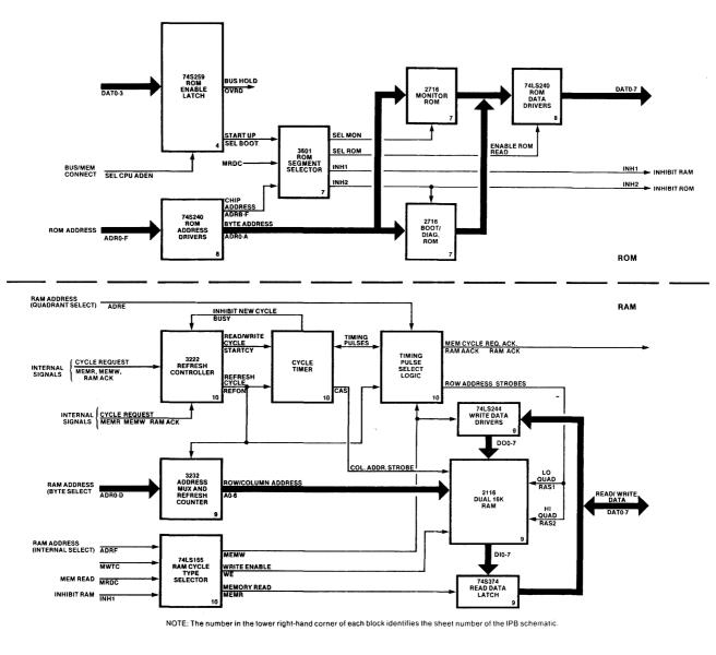
Figure 2-5. IPB Memory Subsystem Block Diagram
