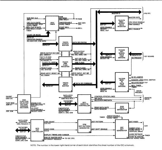
Figure 4-5. IOC I/O Subsystem Block Diagram
