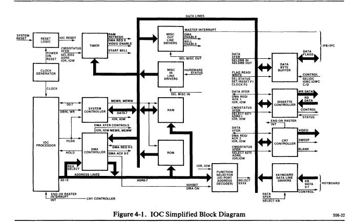
The DBB flags are used to alert the IOC when a command or data byte is input by the IPB/IPC and to indicate when a status or data output byte is accepted by the IPB/IPC. The flags are also used by the IPB/IPC to determine the status of IOC operations. The basic operational sequence of the IOC is as follows:
