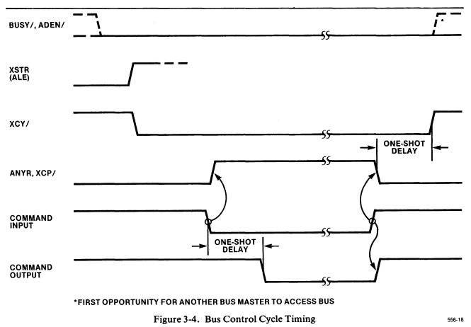
causes ANYR and the corresponding command output to return to an inactive level. The negative transition of ANYR, at the XCP input, triggers the internal delay timer. During the 100 ns hold time interval, ADEN/ and BUSY/, remain active to hold the data bus transceivers enabled and to maintain bus access. (Another bus master can acquire the bus only after the timeout interval). Figure 3-4 illustrates the bus control cycle timing.
