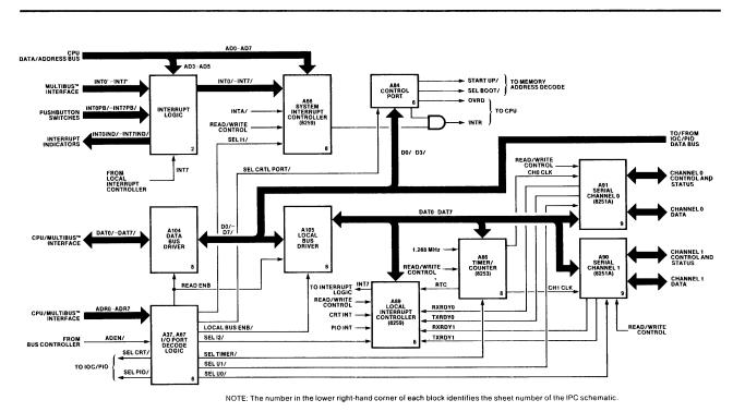
Figure 3-7. IPC I/O Subsystem Block Diagram
