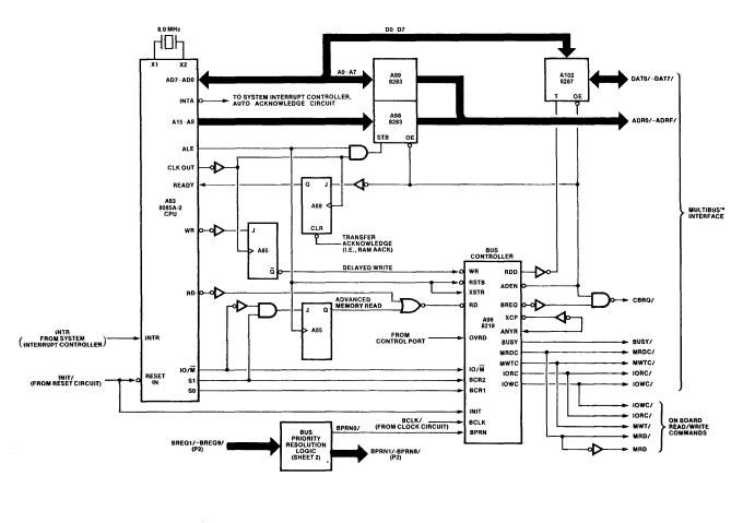
Figure 3-2. Master Processor Subsystem Block Diagram
