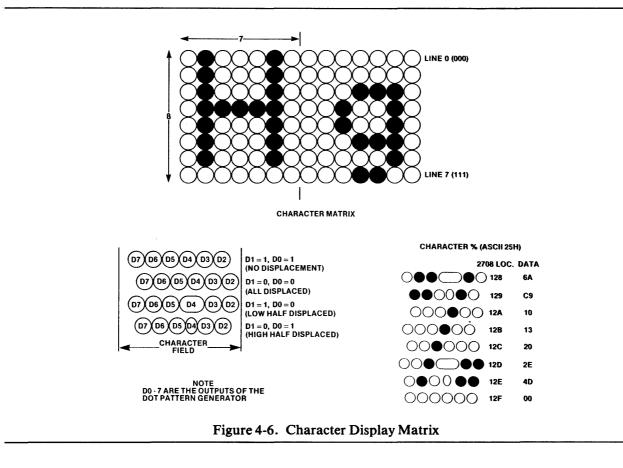
The 6-bit dot pattern and the two displacement bits are output by the character font ROM as a parallel byte. The CRT dot generator serializes the string of dot patterns and inserts the delays specified by the displacement bits. The resulting serial stream of dots is synchronized to the horizontal sweeps and is blanked during retrace time and during the sweeps that separate the rows of characters. Dot pattern timing is shown in figure 4-7.
