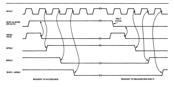
Figure 3-3. Bus Acquisition Timing
