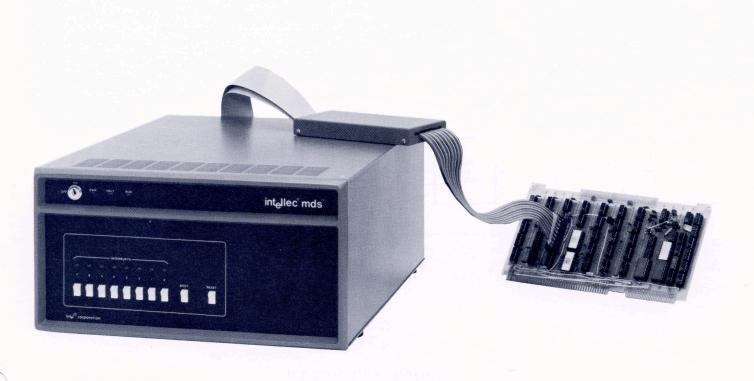
ICE-80 allows the user to assign Intellec MDS resident memory and I/O to the user system. Once assigned, the MDS memory or I/O becomes a part of the user system. The user system may operate with all MDS resident memory and I/O, all user provided memory and I/O, or a combination of both.
