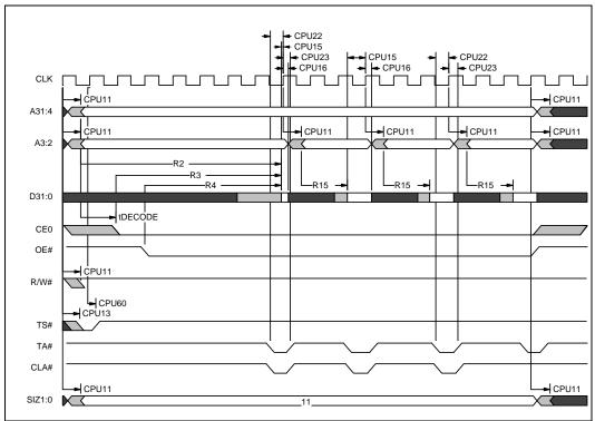
NOTE: The address line labels in this diagram refer to the labels on the 68060. Ax on the 68060 is Ax-1 on 3 Volt Intel<sup>®</sup> StrataFlash<sup>™</sup> memory
