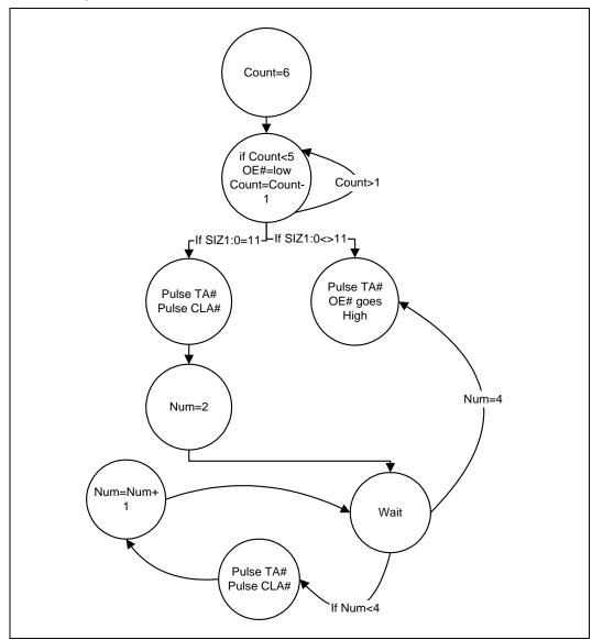
NOTE: Diagram assumes page-mode is enabled and accesses are sequential. Initial wait-states are for 32-Mbit 3 Volt Intel<sup>®</sup> StrataFlash™ memory.
