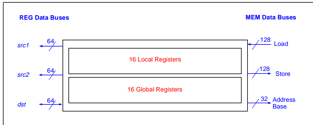
Figure E-4. Six-Port Register File
