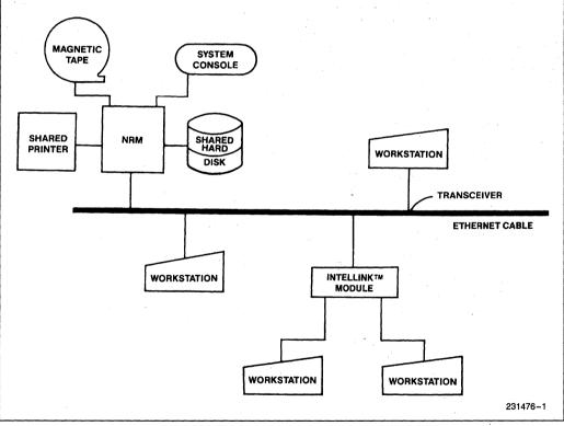
Figure 1. The Network and Its Components
