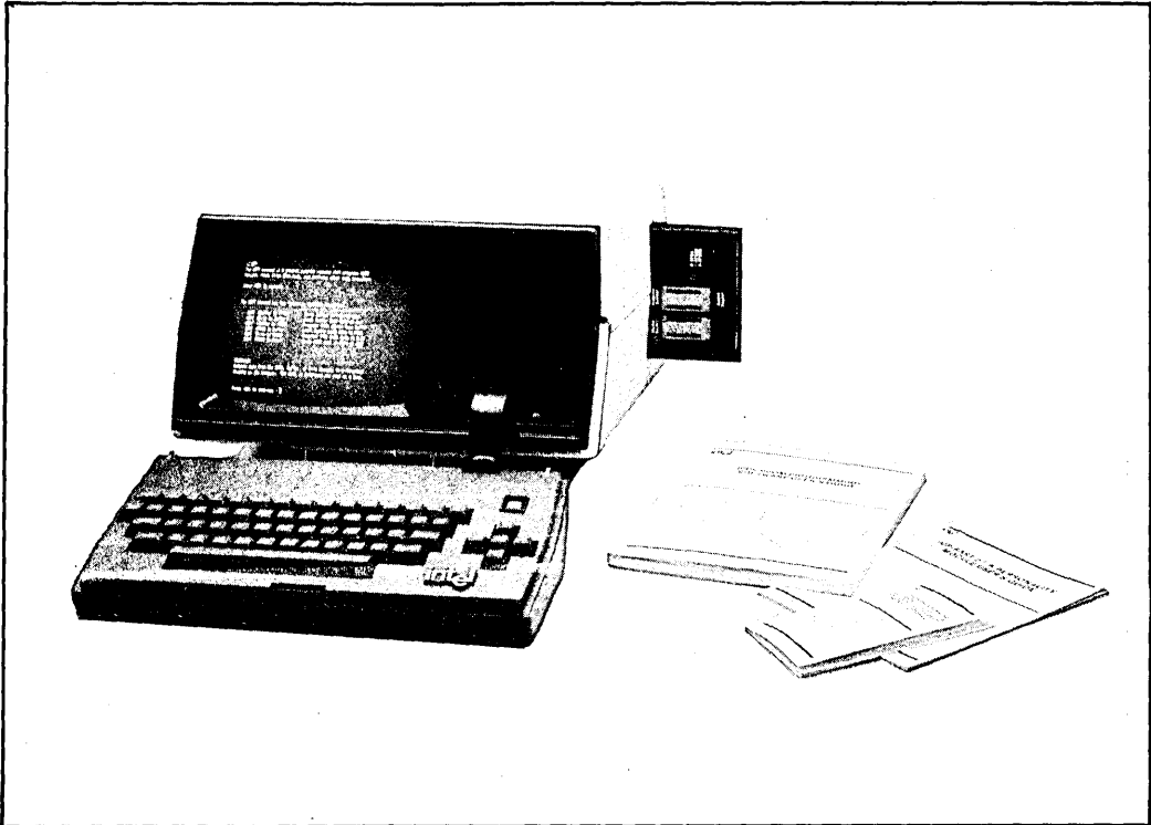
Figure 1 iPDSTM System with PROM Programming Personality Module
