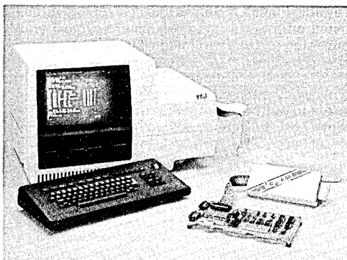
Figure 1. The ICE-85B system hosted by a Series IV development system and connected to a user prototype system.
