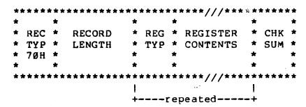
This record provides information about the 8086 registers/register-pairs: CS and IP, SS and SP, DS, and ES. The purpose of this information is for a loader to set the neccessary registers for initiation of execution.
