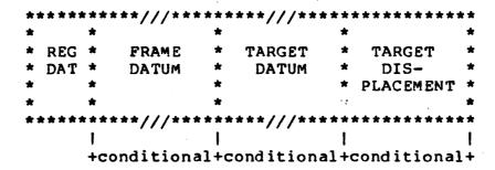
In this case the register contents are specified in exactly the same manner as in the specification of the mapping of a logical address to a physical address as used in the discussion of fixups and the FIXUPP record. The above subfields of the REGISTER CONTENTS field have the same semantics as the FIX DAT, FRAME DATUM, TARGET DATUM, and TARGET DISPLACEMENT fields in the FIXUPP record. Frame method F4 is not allowed.
