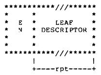
The EN field is a byte: the 8 bits, left to right, indicate if the following 8 Leaves (left to right) are Easy (bit=0) or Nice (bit=1).
