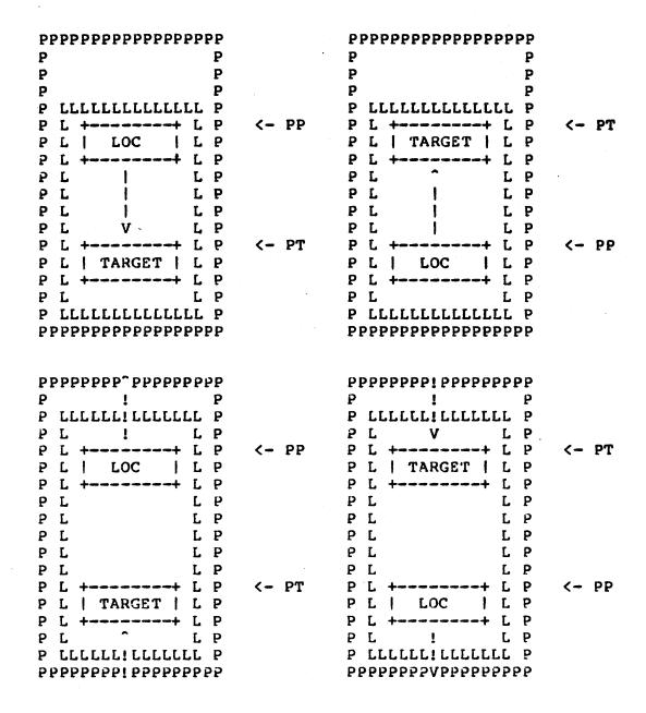
Depending on the absolute length of the arrow, LINK can perform a "normal" fixup or a "clever" fixup (exclamatory arrow). Note that even if the LSEG continues to grow in future LINKing, the fixup is OK as long as the LSEG remains less than 64K in length, which is enforced by LINK. Thus the fixup is completely resolved by LINK.
