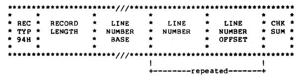
This record provides the means by which a translator may pass to a debugger program, the correspondence between a line number in source code and the corresponding translated code.
