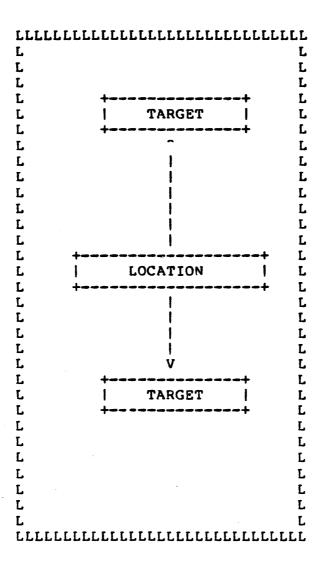
Self-Relative references within a single LSEG do not require a fixup, the translator puts the appropriate value into LOCATION.
