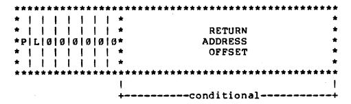
The P (Procedure) bit, if 1, indicates that the BLKDEF record was generated from a procedure in the source. The RETURN ADDRESS OFFSET is present only if P=1.
