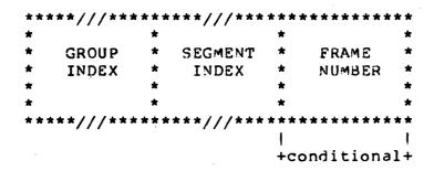
The DATA RECORD BASE specifies the base relative to which the final address of the data record may be defined. It has the same format and interpretation as the LOCAL SYMBOL BASE described for the LOCSYM record.
