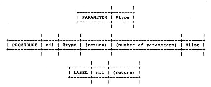
where "(scalar type)" can be either UNSIGNED INTEGER, SIGNED INTEGER, or REAL, "(return)" can be either SHORT or LONG (which indicates, in the case of a LABEL, whether a jump to the label should be a "short" jump or a "long" jump, respectively), and the following values are assigned:
