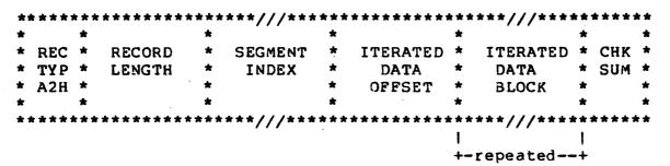
This record provides contiquous data, from which a portion of an 8086 memory image may eventually be constructed. The data will probably NOT be loaded directly by an 8086 loader as it must be further processed by the 8086 R&L products.
