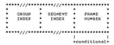
The DATA RECORD BASE specifies the base relative to which the final address of the data record may be defined. It has the same format and interpretation as the LOCAL SYMBOL BASE described for the LOCSYM record.
