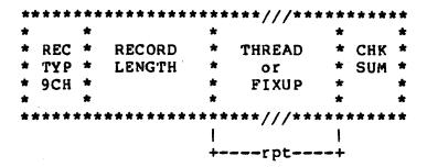
This record specifies 0 or more fixups. Each fixup requests a modification (fixup) to a LOCATION within a previous DATA record. Each fixup is specified by a FIXUP field that specifies 4 data: a location, a mode, a target and a frame. The frame and the target may be specified totally within the FIXUP field, or may be specified by reference to a preceding THREAD field.
