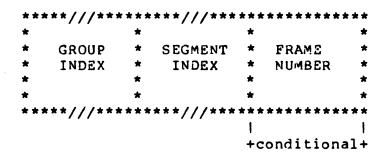
The LOCAL SYMBOLS BASE provides two things: (1) it gives a "referent" value (location in MAS), with respect to which the value (location in MAS) of every symbol in the record will be defined by giving, for each symbol in the record, a non-negative offset; and (2) it gives an indication to LOCATE-86 as to how the final (20-bit) values of the symbols should be decomposed into {base,offset} pairs.
