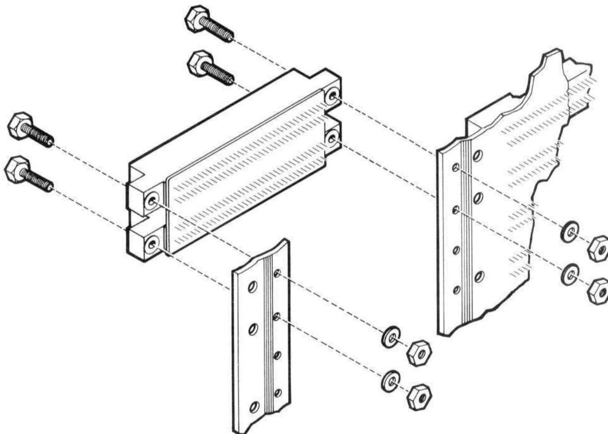
Figure 3. Dual Auxiliary Connector Mounting to Backplane
